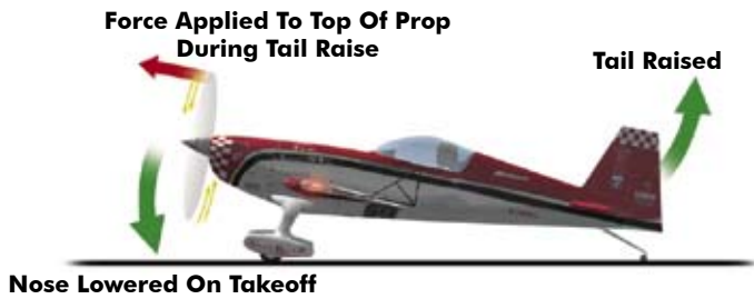
"NOSE LOWERED ON TAKEOFF RUN, FORCE IS APPLIED TO PROPELLER"
