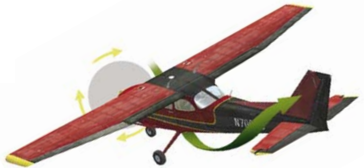
"AIRCRAFT WILL ROTATE OPPOSITE TO PROPELLER ROTATION"
